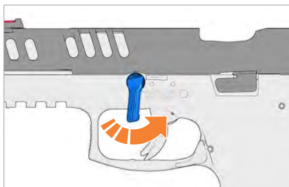
Fig. 68: Turn disassembly lever anticlockwise
