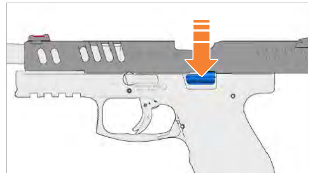
Fig. 20: Press slide release downwards
