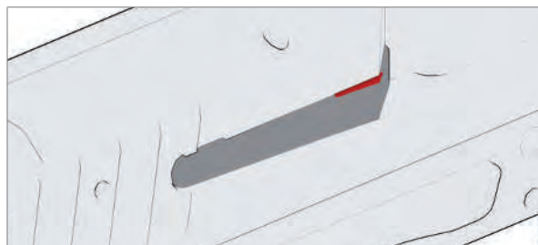
Fig. 12: Loaded chamber indicator
