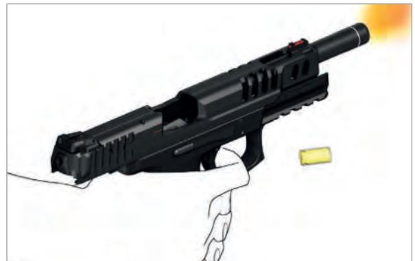
Fig. 53: Path of the slide
